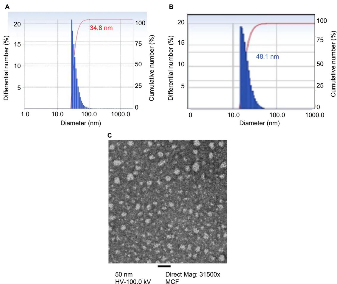
**Figure 1** Particle size measurement by DLS and TEM.
